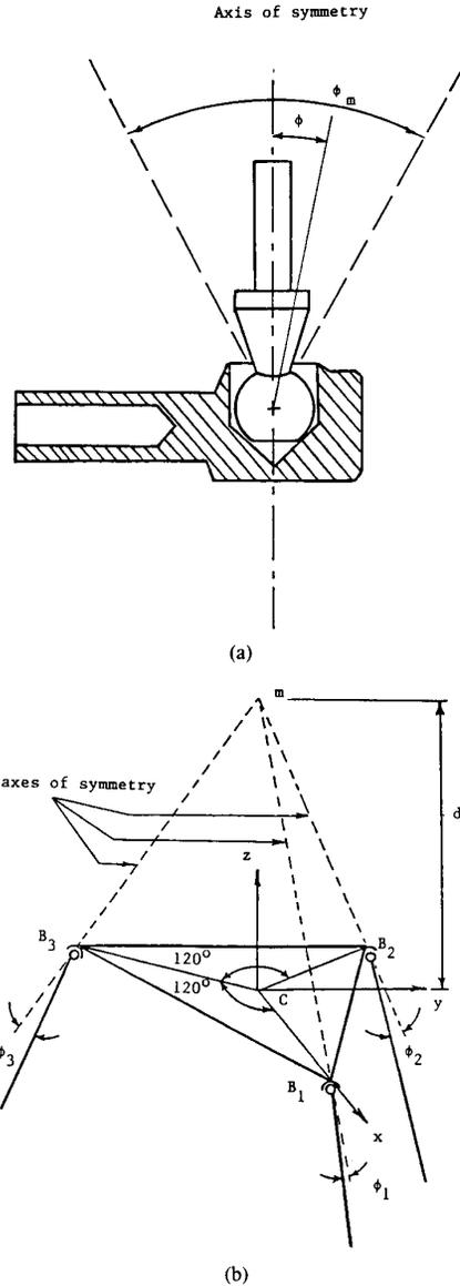
Fig. 3. (a) Ball-joint schematic. (b) Location of ball joints with respect to moving platform.
