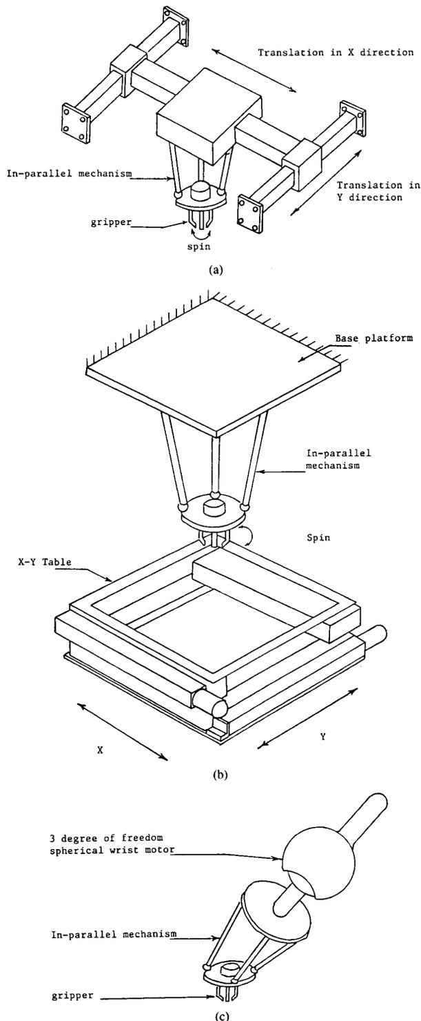
Fig. 6. (a) Schematic of an in-parallel actuated mechanism with moving Cartesian based frame. (b) Schematic of a six-degrees-of-freedom manipulator system which consists of an in-parallel actuated mechanism and an X-Y table. (c) Schematic of a six-degrees-of-freedom end effector based on a combination of in-parallel actuated mechanism and spherical wrist motor.
